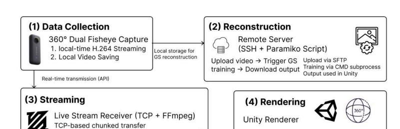
The system has data collection, reconstruction, streaming, and rendering parts to construct remote environments
